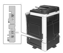
2 Check that a LAN cable is connected to the LAN port of this machine and the green LED is on.
