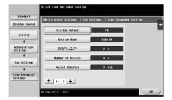
**3** For the push-button type, select [PB], and for the dial-pulse type, select [10pps].
