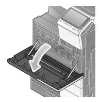
2 Release the Waste Toner Box Lock Lever, then remove the Waste Toner Box.
