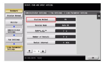
**3** For the push-button type, select [PB], and for the dial-pulse type, select [10pps].
