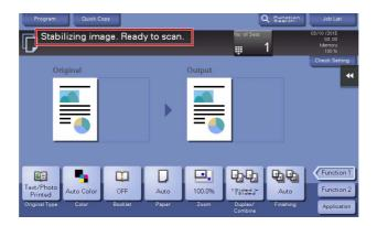
Image stabilization is performed while a large number of copies are being output or the temperature or humidity inside the machine has changed.
