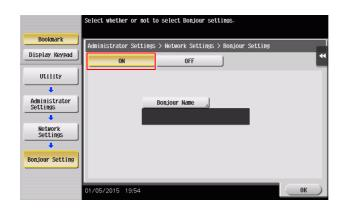
→ The Bonjour name is displayed on the printer driver as a connected device name.
