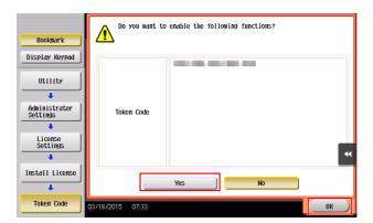
This machine is connected to the Internet to communicate with the License Management Server (LMS), and it restarts automatically.
