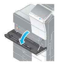
2 Release the Waste Toner Box Lock Lever, then remove the Waste Toner Box.
