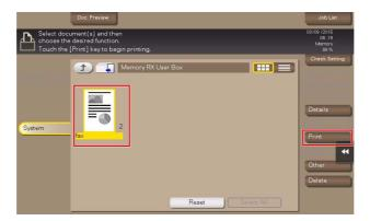
5 Check the message, then tap [Yes]. The fax is printed and automatically deleted from the Memory RX User Box.
