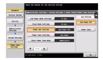
After the setting is changed, the power save mode shifts as shown below depending on how the Power key is pressed.
