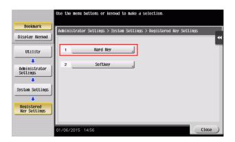
2 Select the [Register key] to be assigned with the voice guidance function.
