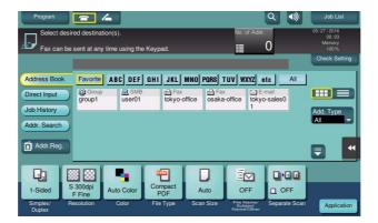
2 Narrow down destinations using index and address type.
